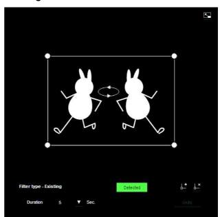
Similar to a active window an trigger area can also be moved and vertexes can be moved/added or deleted. If an object exists within the window longer than the specified time, existing is acknowledged.
